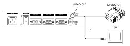
2. Connect the other end of the RCA cable to the RCA input port on the projector or TV.
